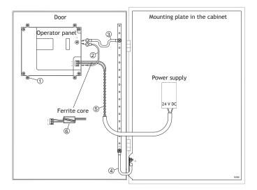
The operator panel's mounting clamps do not provide a secure grounding connection between the panel and the device cabinet, see 1 in drawing above.
