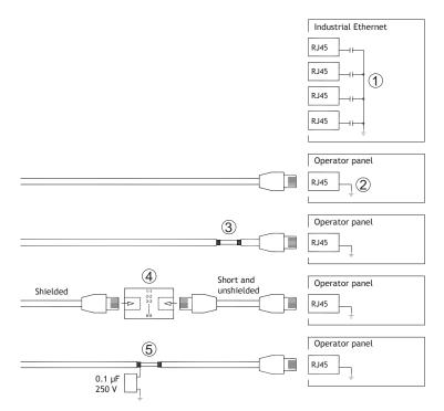
In some industrial units for Ethernet, the RJ45 contact's shield is connected to the chassis via a capacitor, see 1 in drawing above.
