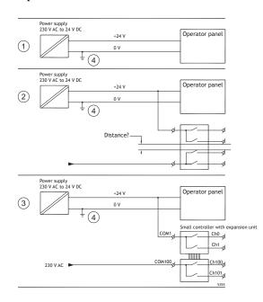
If a power supply that meets safety standards is used and only feeds the operator panel, there is no problem. See 1 in drawing above.
